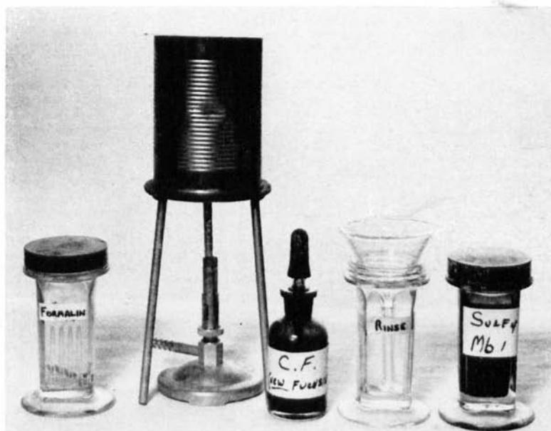
Fig. 3. Materials and arrangement for fixation and staining of films.
