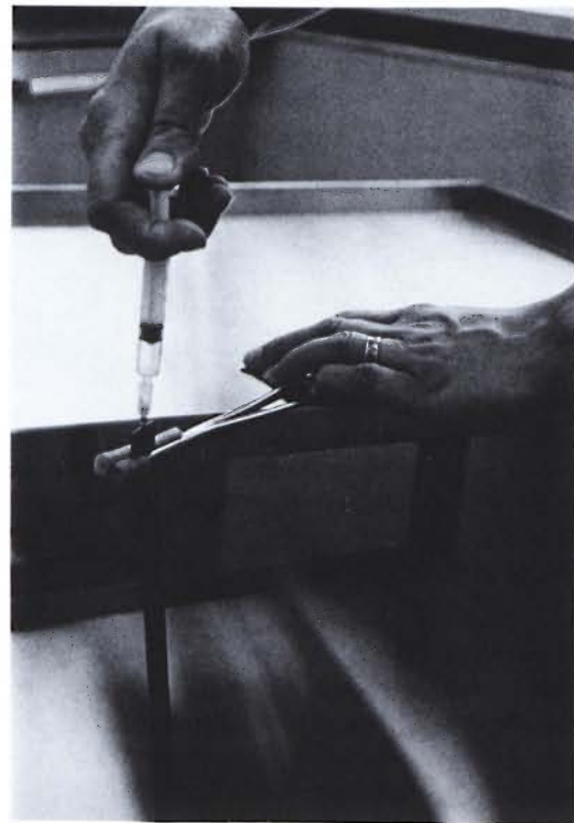
FIG. 4. Method of injecting monobath to develop filmstrip, showing plastic envelope with filmstrip.
