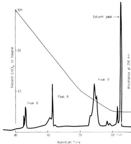
FIG. 2. Adsorption chromatography of fatty acids with more than 1000 molecular weight. Elution was performed with a linear gradient of CHCl<sub>3</sub> from 0–30% in n-hexane. The flow rate was fixed at 1 ml/min.
