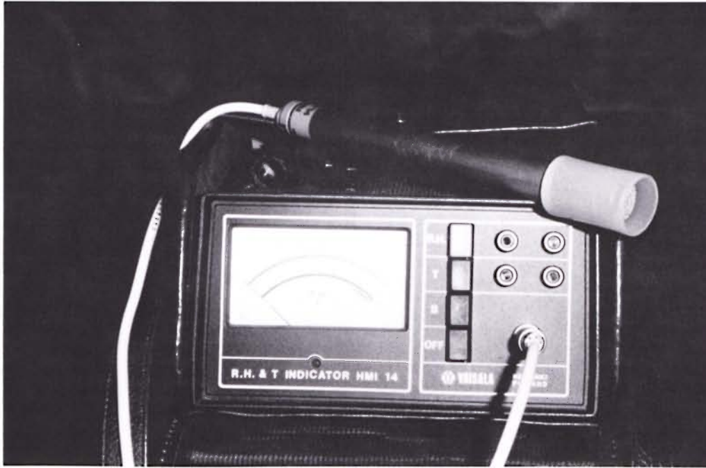
FIG. 1. The indicator and probe of the Vaisala Humicap humidity meter. Probe is equipped with a cylindrical plastic hood.
