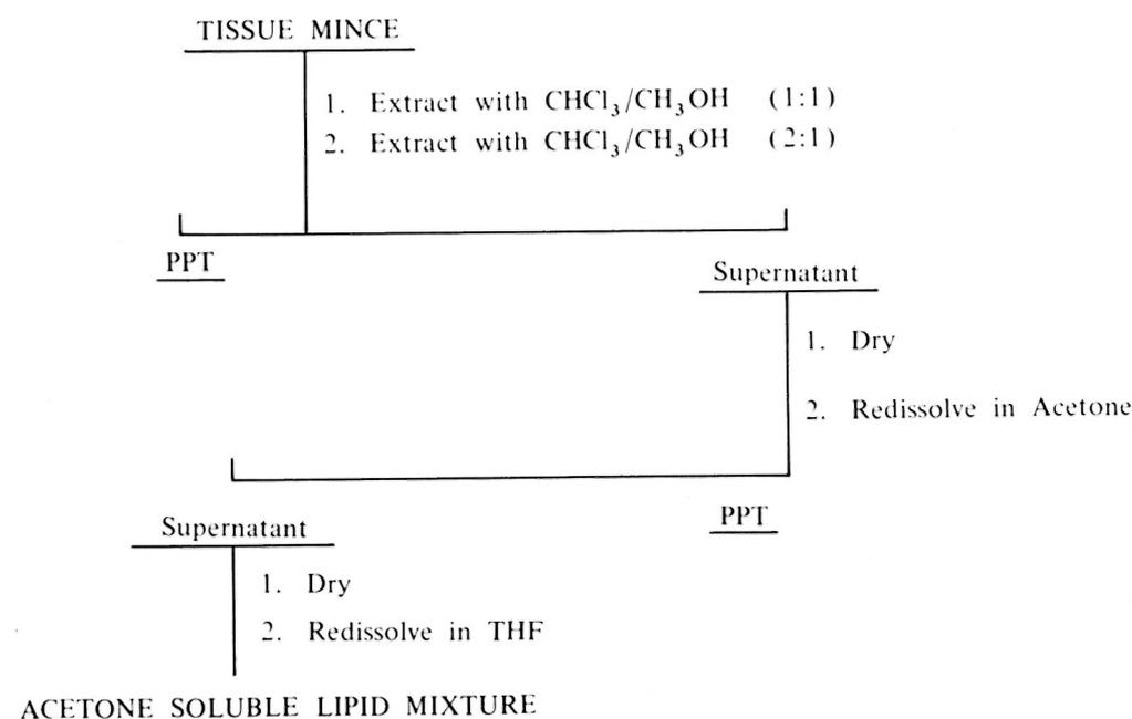
FIG. 3. Procedure for extraction of acetone soluble lipids.
