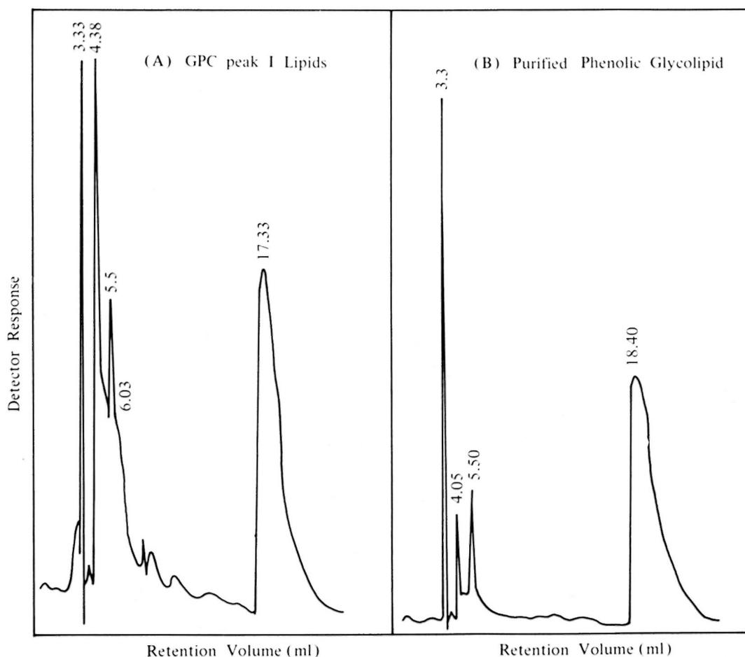
FIG. 5. Normal-phase (SILICA) analysis with spectrophotometric detector at 280 nm wavelength.
