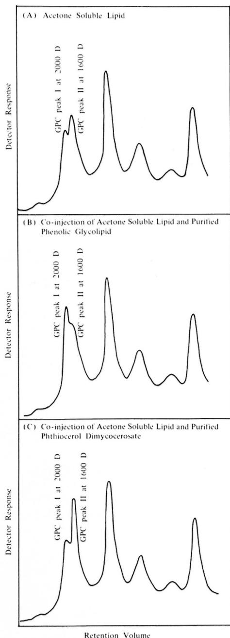
FIG. 4. Gel permeation chromatography (GPC) (Shimadzu-HSG) analysis with RI detector.
